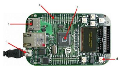
Figure 5.5 The LM3S6965 prototyping board: a) ARM® Cortex-M3 Processor, b) GPIO port for output digital data, c) USB port for system programming and debugging, and for connecting User interface when in running mode, d) Reset button, e) Memory card slot for extra data and program storage.
